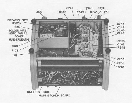
Figure 8. Bottom interior view of the Type 1232-A.
