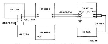
Figure 7. Filter Tuning Dial Test Set-up.
