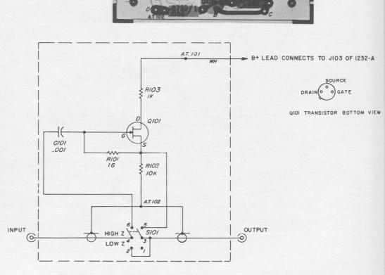
Figure 14. Schematic diagram and etched board layout of the Type 1232-P2 Preamplifier. The etched board part number is 1232-2730.
