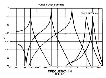
Figure 3. Typical filter characteristics of the Type 1232-A.
