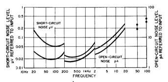
Figure 6. Typical noise levels as a function of frequency.
