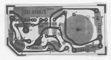
Figure 13. Etched Board Layout of the Type 1232-A Tuned Amplifier and Null Detector, P/N's 1232-2700 and 1232-2710.
