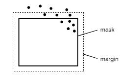
Figure 16.2. Mask with Positive Margin. (8 total hits, 3 margin hits, 5 mask hits)
