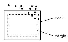
Figure 16-3. Mask with Negative Margin. (6 total hits, 4 margin hits, 6 mask hits)
