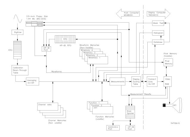
The cal table automatically applies the calibration factors to the raw data, so that the output of the cal table is calibrated data.
