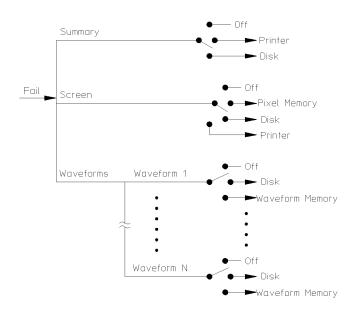
Mask Test Subsystem Functional Diagram
