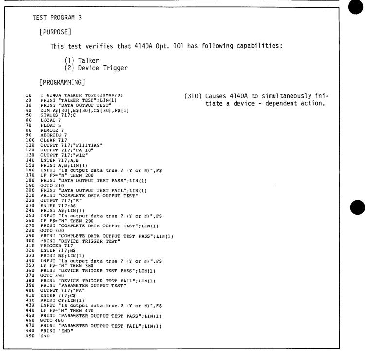
Figure 4-12. HP-IB Interface Test Program 3 Using 9835A.
