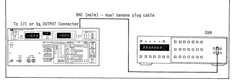
Figure 4-8. Analog Output Accuracy Test Setup.
