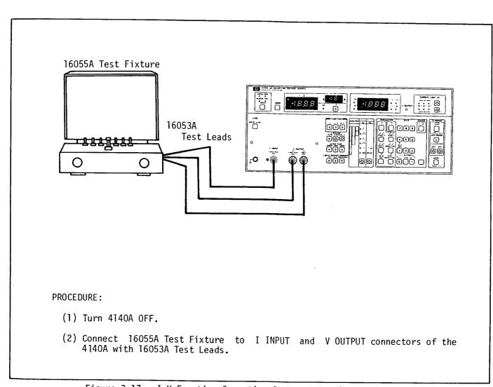
Figure 3-17. I-V Function Operating Instructions (sheet 1 of 4).
