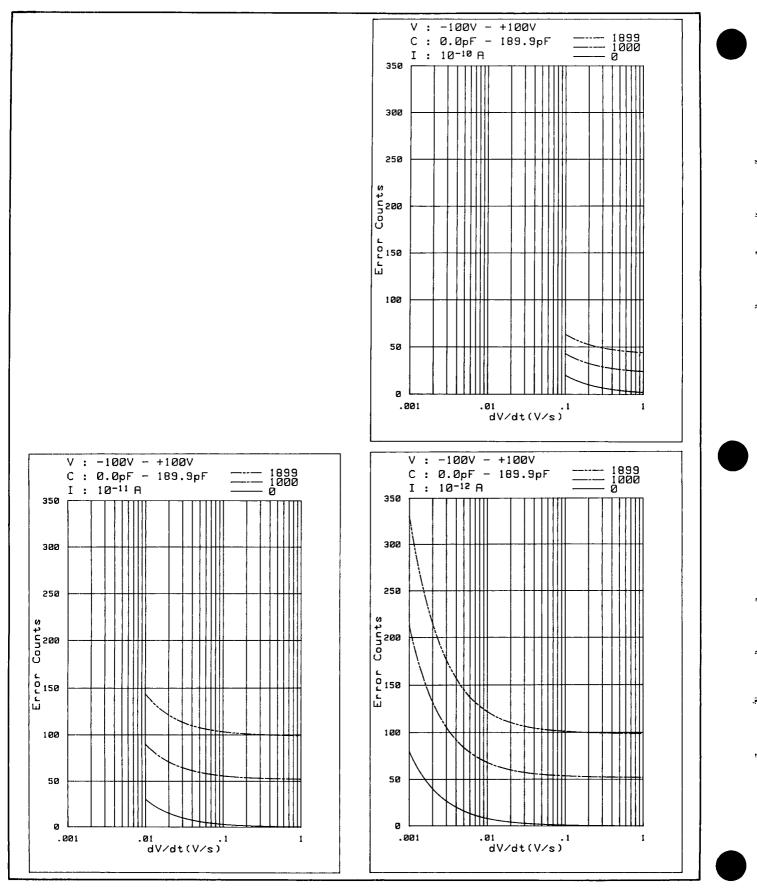
Figure 3-22. C-V Measurement Accuracy (Sheet 3 of 4).
