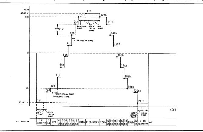
Figure 3-8. Relationship between Output Voltage and Display for A. (Double Staircase Wave).
