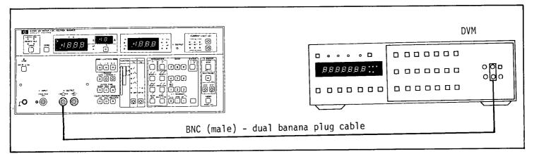
Figure 4-5. Ramp Wave Start Voltage Accuracy Test Setup.
