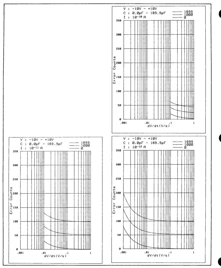
Figure 3-22. C-V Measurement Accuracy (Sheet 1 of 4).
