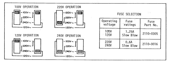
Figure 2-1. Line Voltage and Fuse Selection.
