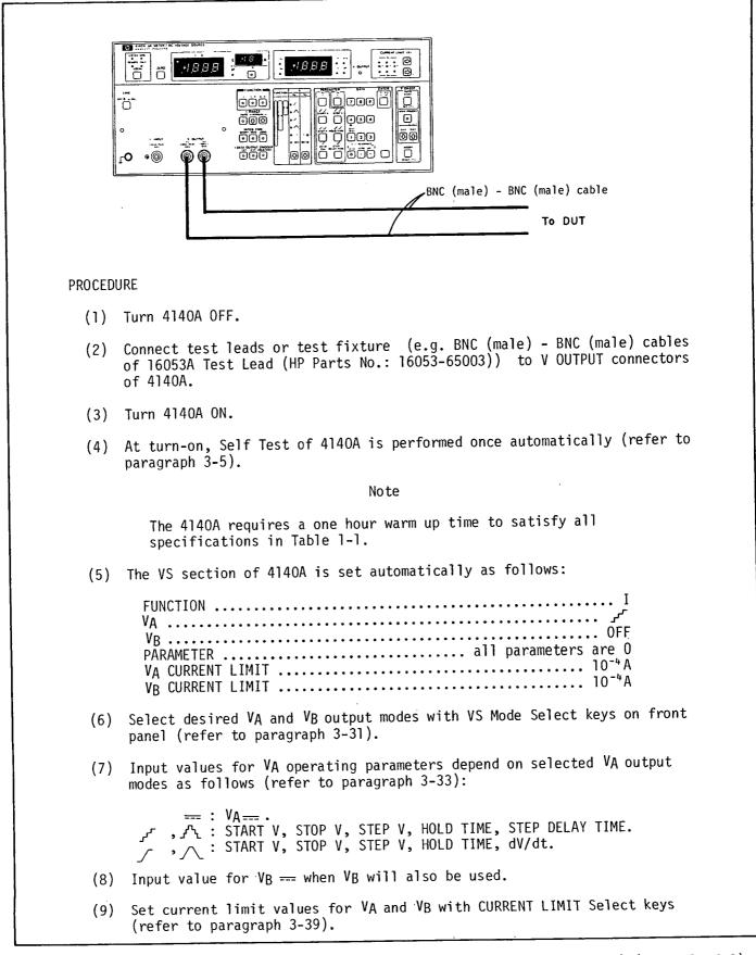
Figure 3-12. VS Section Operating Instructions (when FUNCTION is set to I) (sheet 1 of 2). 3-20
