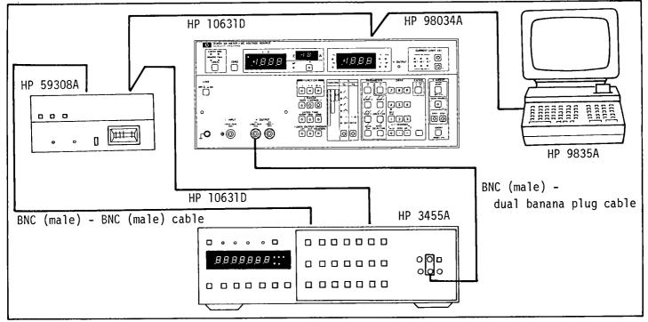
Figure 4-6. Ramp Rate Accuracy Test Setup.
