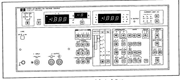
Figure 3-3. Octal Codes of Control Keys.
