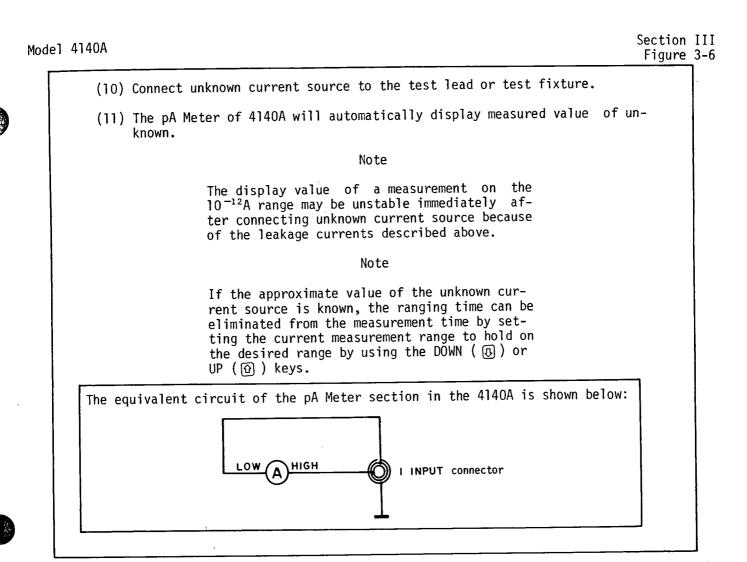
Figure 3-6. pA Meter Section Operating Instructions (when FUNCTION is set to I) (sheet 2 of 2).
