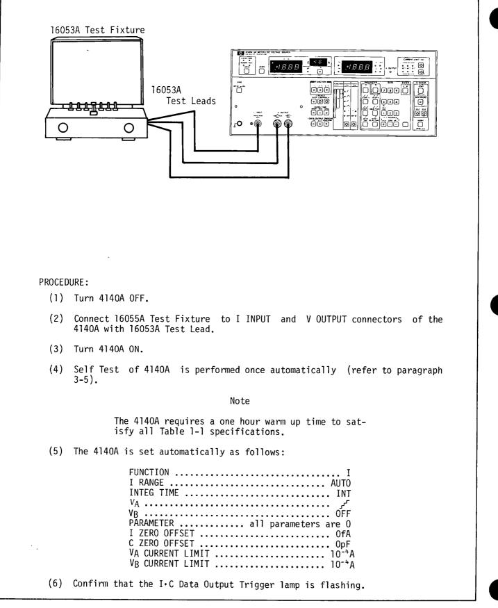
Figure 3-23. C-V Function Operating Instructions (sheet 1 of 3).
