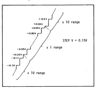
Figure 3-11. Output Voltage Range of Staircase Wave.
