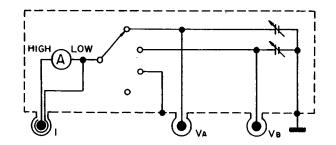
16055A: Test Fixture for General Device Measurements
