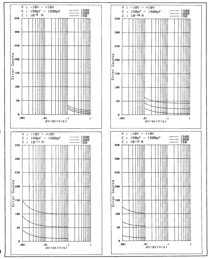
Figure 3-22. C-V Measurement Accuracy (Sheet 2 of 4).
