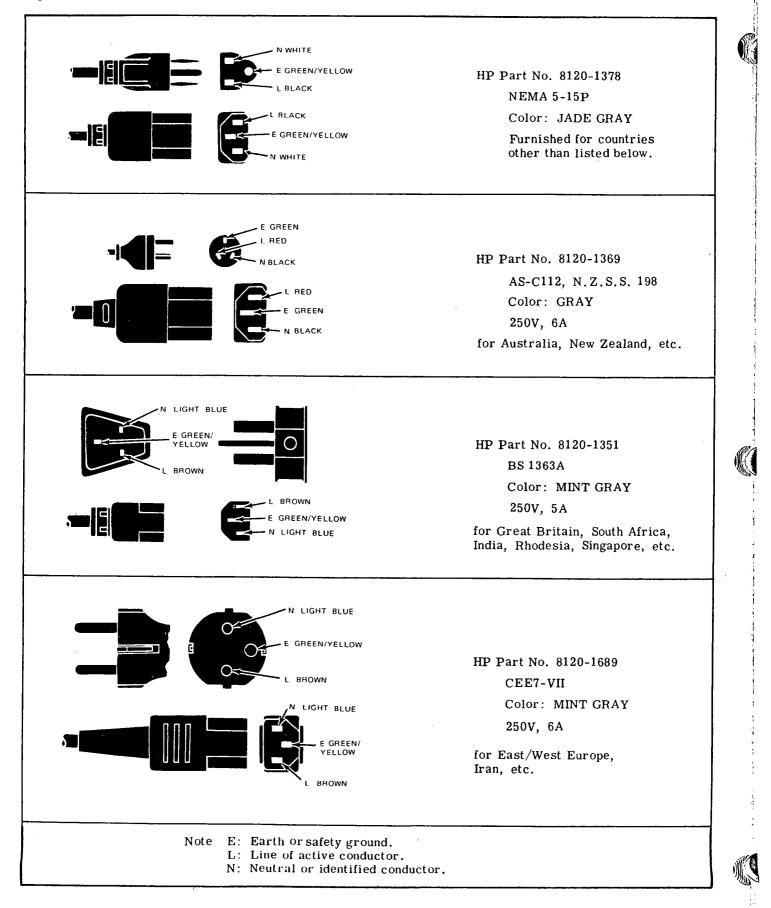
Figure 2-2. Power Cables Supplied.
