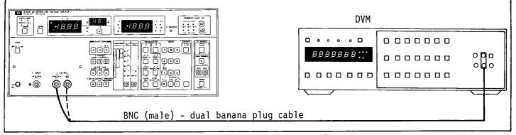
Figure 4-1. Voltage Output Accuracy Test Setup.
