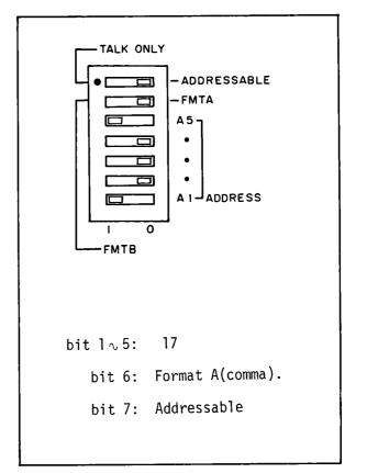
Figure 3-25. HP-IB Control Switch.
