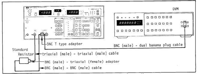
Figure 4-3. Current Accuracy Test Setup ( $10^{-8} A \circ 10^{-12} A$  Ranges).
