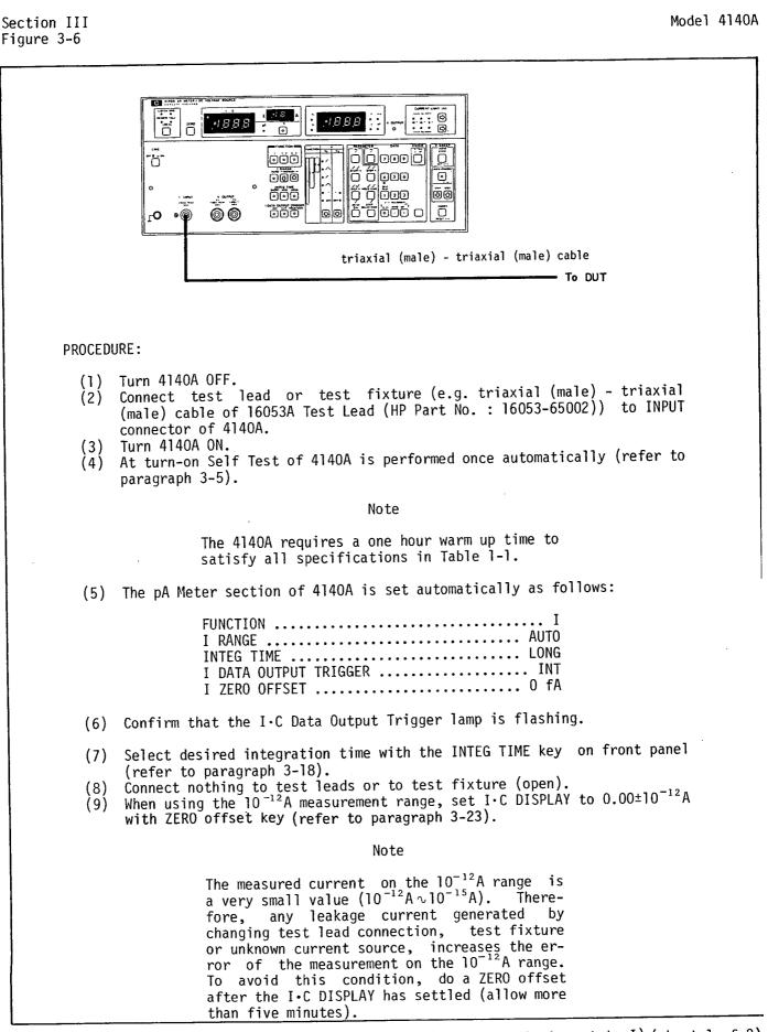
Figure 3-6.pA Meter Section Operating Instructions (when FUNCTION is set to I) (sheet 1 of 2)
