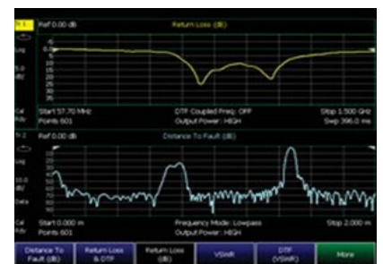
View return loss and DTF simultaneously
