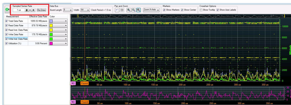
Figure 3. Customize performance views by changing sample rate and performance measurement selections.
