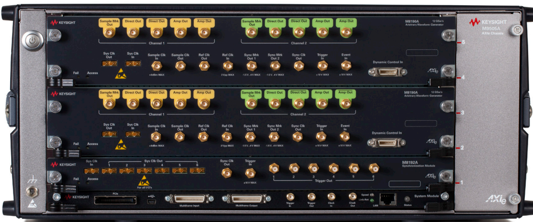
Five slot AXle chassis with two M8190A AWG; can contain an embedded controller.
