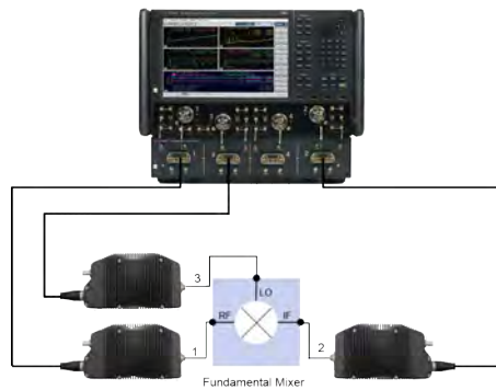
A dual-source PNA with an N5292A four-port controller and broadband frequency-extender modules characterize mixers and converters at millimeter wave frequencies. The PNA's second source can be used to provide an LO signal to a mixer.
