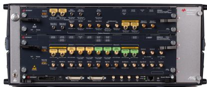
Figure 29. Overview of possible J-BERT M8020A configurations.
