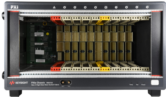
Figure 1. M9010A 10-slot PXIe Gen 3 chassis
