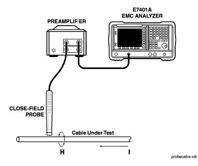
Use the close field magnetic probe to determine the magnetic field intensity around a cable. The current density can then be calculated if the distance from the center of the cable to the center of the probe loops is known.
