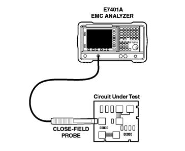
A close field probe like the Agilent 11940A or 11941A is a useful tool for locating susceptible circuits. The probe is driven from a signal generator tuned to a problem frequency, and then is moved along the circuitry until a problem is located. The relatively small size of a probe enables the isolation of the problem. If the frequency of the problem is not known, use a swept source like the tracking generator of a EMC analyzer.
