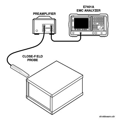
Use the close field probes to isolate gaps in shield and electrical gaskets. Even loose screws can cause a problem. A quick evaluation procedure involves placing the display of the analyzer in **Max Hold** mode to collect the strongest emissions found among repeated sweeps. Scanning the close-field probe along the seam records the worst-case values. This result is then saved, and the analyzer display is returned to **Clear Write** mode so that the strongest source of emissions can be located.
