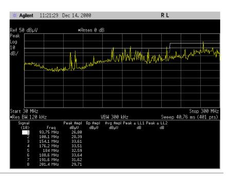
When the automeasure process in complete, the emissions above the limit line margin will be displayed in the signal list with the measured peak amplitude.
