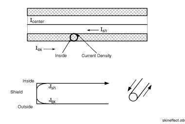
At low frequencies the current is evenly distributed throughout the conductor. But at higher frequencies, the skin effect enables the cable shield to provide additional protection. Here, most of the return current flows on the inside of the shield because it is the surface closest to the center conductor in which the signal current flows.
